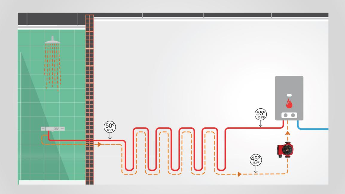
Energy wasted with continuous recirculation in DHW
